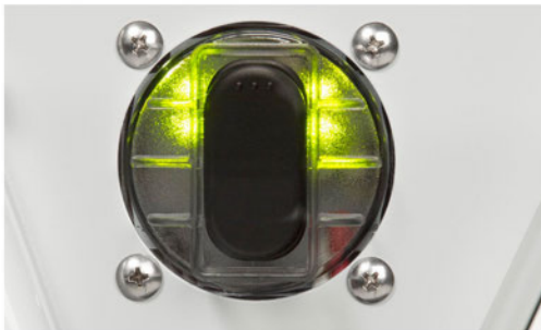
1. In FULL POWER mode - PRESS ON - the lights around the switch will be solid green. In BATTERY SAVER mode - PRESS ON,OFF, ON - the lights will flash green.
