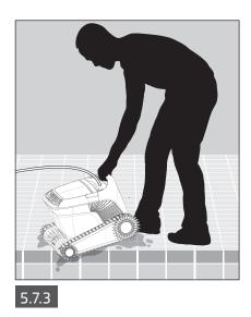
Place the robotic pool cleaner on the edge of the pool and let the water drain out before lifting.
