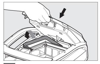
6.2.6 Reposition the inner net basket, check that each filter was placed well, and insert the clean filter basket. Close the filter cover.
