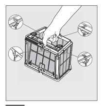
6.2.5 Assemble the filter panels in the following order: Panel 4 —> 3 —> 2 —> 1.
