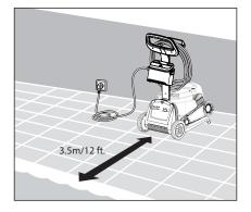
**5.1.1** Position the power supply at approximately the middle of the long side of the pool, at least at a distance of 3.5 m (12 ft).
