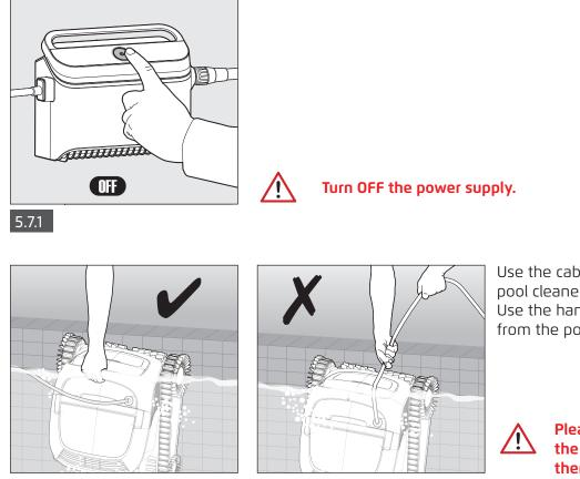
Use the cable to pull the robotic pool cleaner to the side of the pool. Use the handle to remove the robot from the pool.
