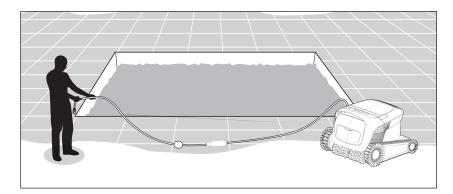
5.1.2 Unwind the cable to ensure that it has no kinks.
